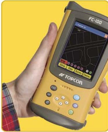
Topcon's Pocket-3D GPS field controller software was designed to be easy to learn and use without sacrificing power and performance. Pocket-3D is the human interface to unlock the power of real time GPS (RTK) positioning on your project site. With accuracies within a couple hundredths of a foot, Pocket-3D combined with Topcon's advanced GPS+ technology provides the perfect job site staking and grade control tool with almost limitless potential.
